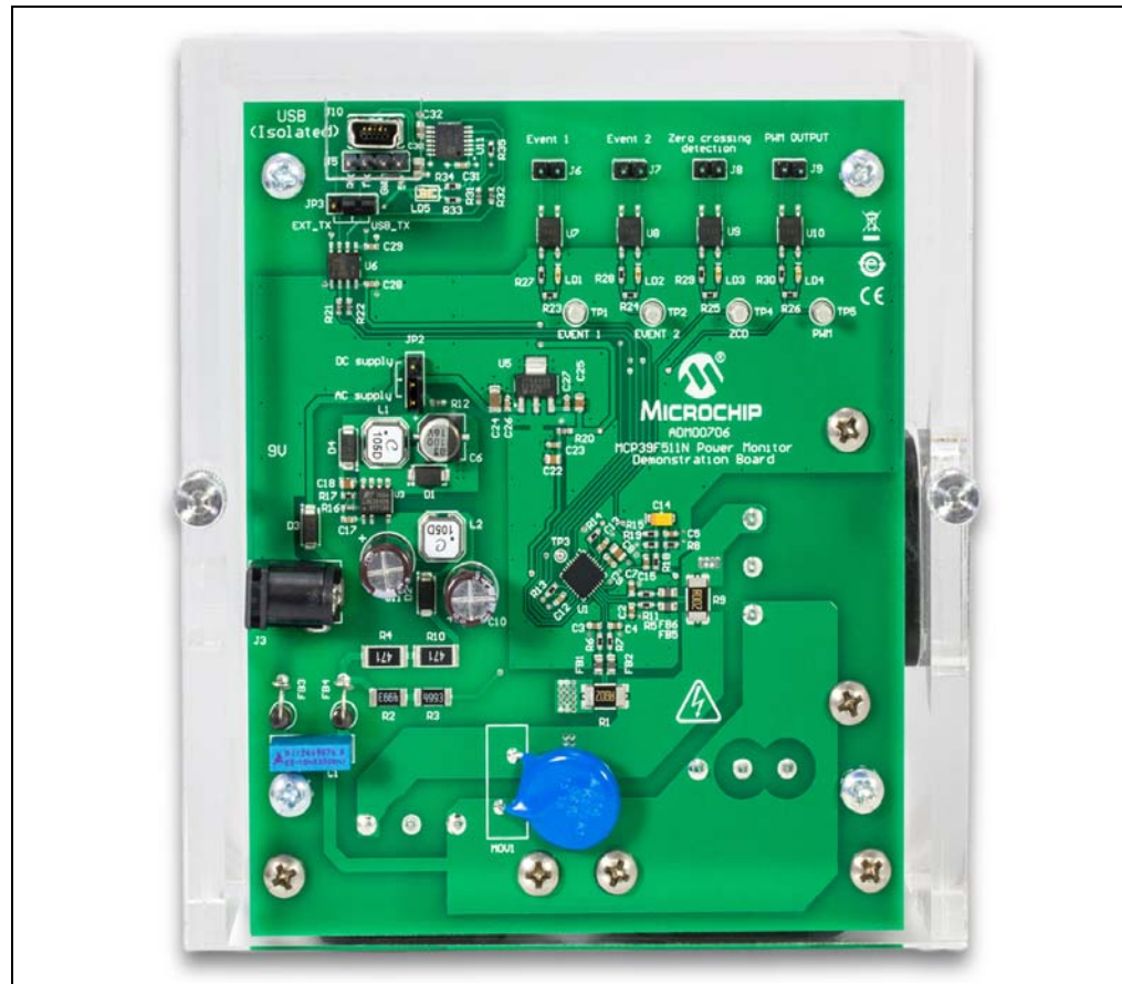
FIGURE 1-1: MCP39F511N Power Monitor Demonstration Board.
