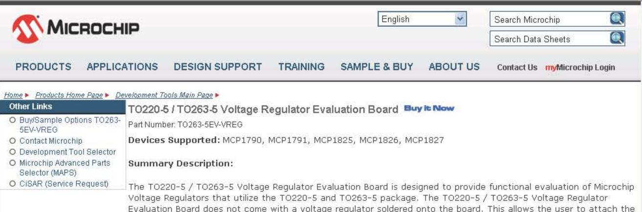
Voltage Regulators that utilize the TO220-5 and TO263-5 package. The TO220-5 / TO263-5 Voltage Regulator Evaluation Board does not come with a voltage regulator soldered onto the board. This allows the user to attach the voltage regulator of their choosing to the board and perform quiescent current, ground current, PSRR, and other desired tests.
