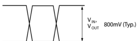
Figure 1a. Single-Ended Voltage Swing
