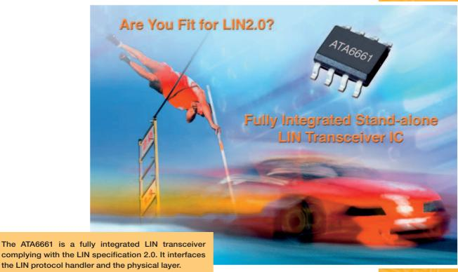
the LIN protocol handler and the physical layer. The device is designed to handle the low-speed data communication in vehicles, for example, in convenience electronics with data transmissions up to 20 Kbaud. In order to comply with the 42V PowerNet requirements, the bus output is capable of withstanding high voltages. Sleep mode guarantees minimal
