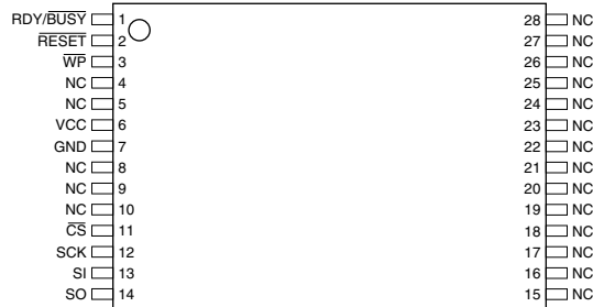
TSOP Top View – Type 1
