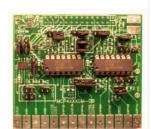
The board also has a voltage doubler device (TC1240A), which can be used to show the WiperLock Technology feature of the MCP4021.
