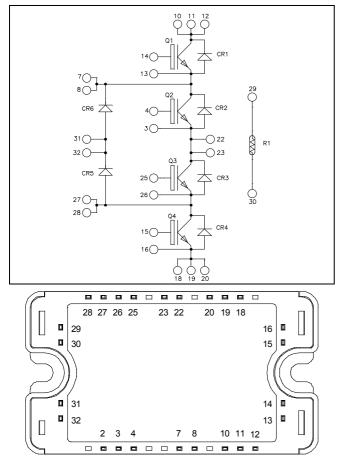
All multiple inputs and outputs must be shorted together Example: 10/11/12 ; 7/8 ...
