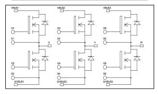
$$\begin{split} V_{DSS} &= 600 V \\ R_{DSon} &= 35 m \Omega \ max \ @ \ Tj = 25^{\circ} C \\ I_D &= 72 A \ @ \ Tc = 25^{\circ} C \end{split}$$
