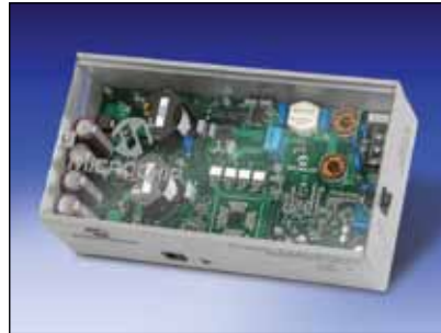
Grid Connected Solar Micro Inverter Reference Design
