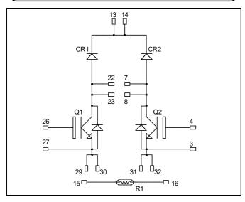
All multiple inputs and outputs must be shorted together Example: 13/14; 29/30; 22/23 ...
