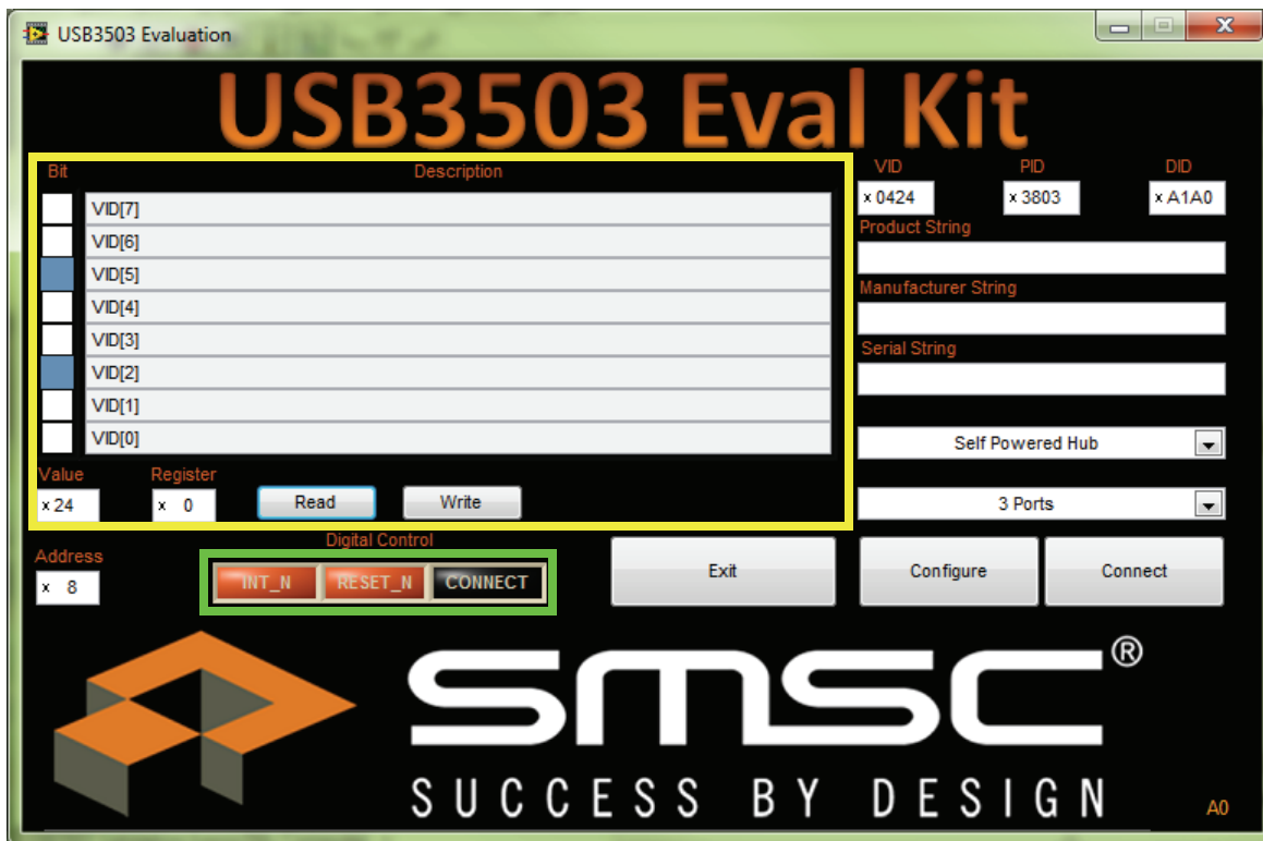
Figure 4.3 Digital Control (Green) and I 2 C (Yellow) Sections
