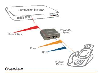
PowerDsine's PD-AS-701 High-Power active splitters enable data terminals that were not originally designed to accept power from the Ethernet, to be powered by HiPoE (High Power over Ethernet) switches and midspans. The PD-AS-701 High Power series (12v, 18v and 24v) can power devices such as WiMAX CPEs, small WiMAX base-stations, 802.11n Access-Points, Thin-Clients, Video-Phones, PTZ (Pan/Tilt/Zoom) IP Cameras and more.
