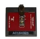
Part Number: AC164325 - MPLAB PM3 Socket Module for 8L MSSOP
