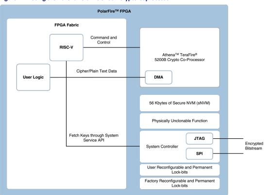
Figure 12 • Using the Athena TeraFire 5200B Crypto Coprocessor
