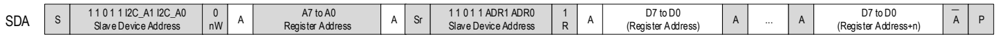
Figure 4. I 2 C Read Data (Slave Transmit, Master Receive) From Any Register Address
