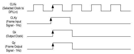
In Figure 8, CLKx is the associated input clock and CLKy is the frame pulse, and they are both input to DPLLn. Qx is the output clock that is locked to CLKx, and Qy is the output frame pulse output of DPLLn.
