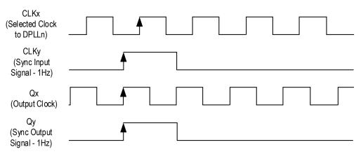
In Figure 9, CLKx is the associated input clock and CLKy is the sync pulse, and they are both input to DPLLn. Qx is the output clock that is locked to CLKx, and Qy is the output sync pulse output of DPLLn.
