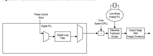
To assist in the above, there is an optional timer associated with the PCW. This allows a phase control word to be applied for a limited period of time after which it will be automatically reset to zero or placed into holdover by the 8A34041, and therefore, it will avoid the DCO continuing to apply the phase adjustment indefinitely until it reaches its tuning range limits. The timer value is a 16-bit integer that has a granularity of 1 millisecond and a full range of up to 65.535 seconds.
