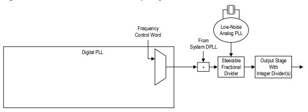
The FCW is a 42-bit 2's-complement value. The FCW has a granularity of  $1.11 \times 10^{-10}$  ppm and a full range of +244.20ppm to -244.08ppm of the nominal DCO frequency. A positive value will increase the output frequency and a negative one will decrease the output frequency. The formula for calculation of the FCW from the fractional frequency offset (FFO) is:
