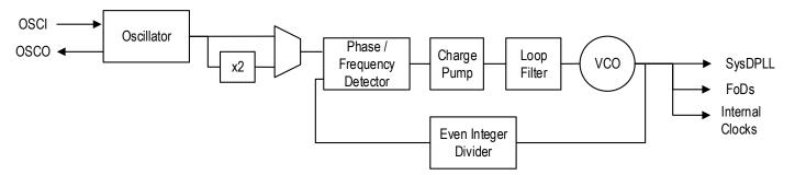
During a device reset, the APLL is configured by loading the appropriate control register fields from the internal One-Time Programmable memory or an external serial EEPROM, whichever is enabled and has valid contents. After the reset sequence has completed, the APLL can be re-configured manually over the serial port at any time.
