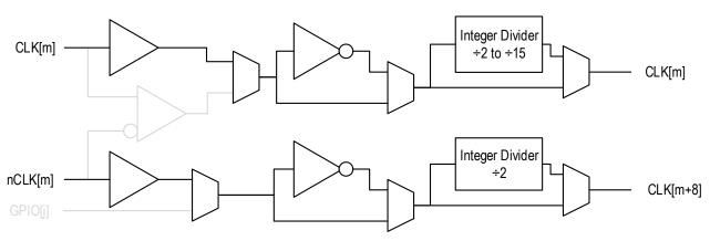
When programmed as differential plus one single-ended as shown in Figure 7, two independent inputs are provided to the 8A34041. This mode can only be used with the GPIOs and input stages shown in Table 5.
