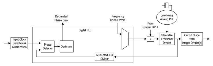
In this case, the phase error measured by the DPLL's phase detector is digitized and decimated to a user selected update rate and provided via registers for use by an external digital filter (for information, see Digital Phase Locked Loop (DPLL)). That data is read from the 8A34041 and provided to the digital filter algorithm. That algorithm then generates a Frequency Control Word (FCW) and writes that back into 8A34041's registers. The FCW will provide direct control of the steerable FOD.
