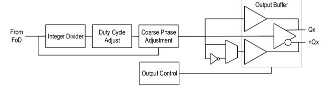
Other than having two copies of each functional block fed from the same FOD, both single and dual output stages behave the same. Similarly, the two paths within the dual output stages behave the same as each other. Descriptions of each functional block are provided in the following sub-sections.
