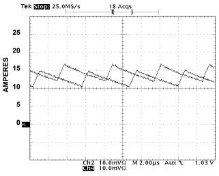
FIGURE 10. TWO CHANNEL MULTIPHASE SYSTEM WITH CURRENT BALANCING ENABLED
