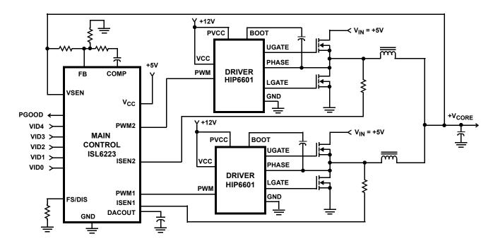
Typical Application - Two Phase Converter Using HIP6601 Gate Drivers
