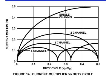
The current from multiple channels tend to cancel each other and reduce the total ripple current. Figure 13 gives the total ripple current as a function of duty cycle, normalized to the parameter (Vo)/(L  $\cdot$  F<sub>S</sub>) at zero duty cycle. To determine the total ripple current from the number of channels and the duty cycle, multiply the y-axis value by (Vo)/(LxF<sub>SW</sub>).
